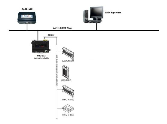
**Note**: Level 9 Microsmart controllers cannot be addressed above address 62. The Level 9 Microsmart controllers must reside on the first 62 addresses. They will not communicate above address 62. This is a Level 9 Microsmart device limitation. If more than 62 Level 9 Microsmart devices exist, break up the network into two trunks and use two Microsmart drivers and RS-485 trunks.
