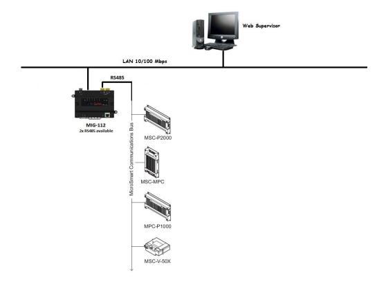
Options 2 - (Microsmart N4 driver will install at the JACE and communicate to the MIG-112 gateway controller).
